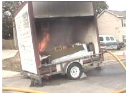
Sprinklered bedroom fire at time of sprinkler activation
