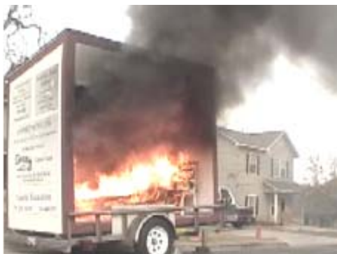
Fire in demonstration trailer (no sprinklers)
